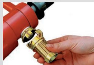
**DK09: Coupling exhaust adapter for dry drilling**
