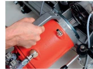
With my saw blade of 750 mm diameter I cut concrete walls and masonry up to 320 mm deep without taking care of reinforcement.
