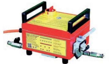
My converter recognizes, if I am connected to 230 V or to 400 V and adapts current and power accordingly. My motor current is controlled according to the requirements and limited to the maximum. Thus I can not be overloaded. The temperature of my motor is checked constantly. If I am loaded too much or cooled too less, my power electronic switches me off before anything can happen. Status and error signals are indicated to the user via an LED mounted on the frequency converter.
